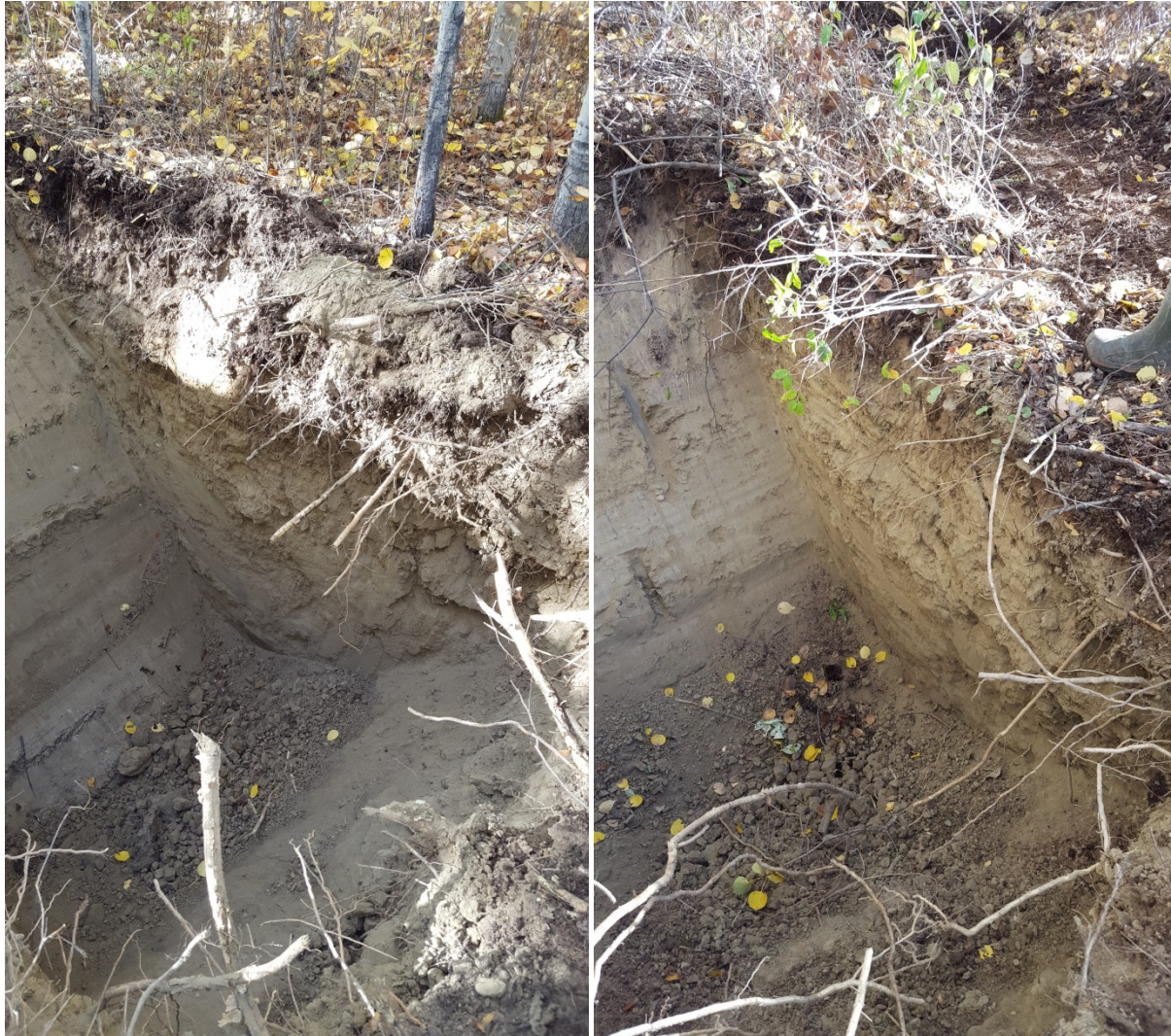
Figure 5/6 Showing Observation holes for the Lots B and C respectively. Soil remains consistent throughout
