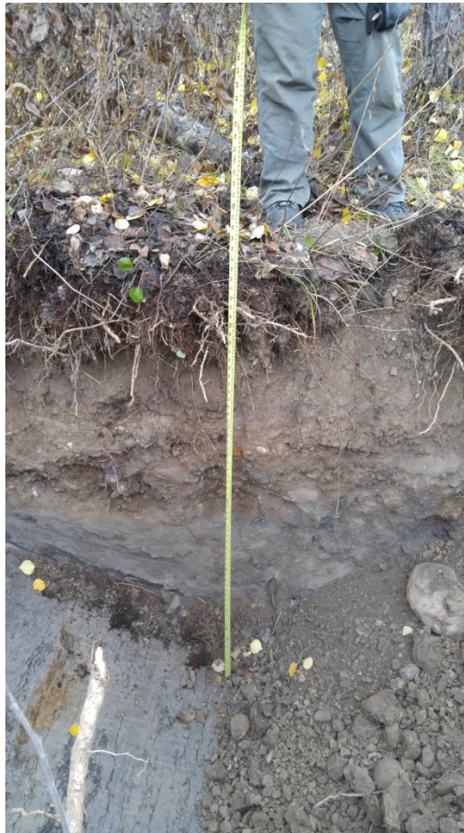
Figure 7: Remainder Lot 3 observation hole. 5 inch of top soil, 15 inch of clay and 33 inch of shale
