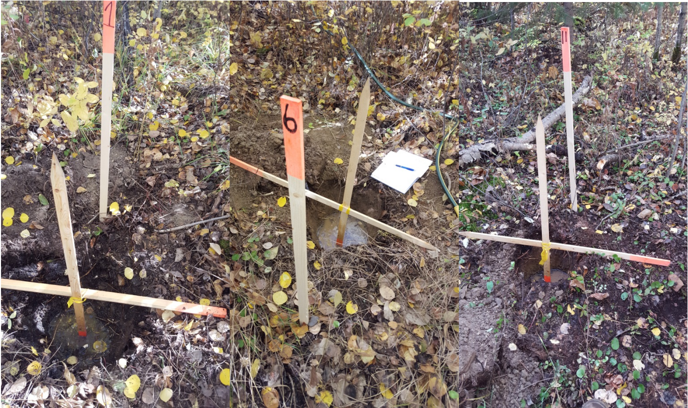
Figure 2/3/4: Showing holes used for percolation tests. Photos are for lots B, C and Remainder Lot 3 respectively
